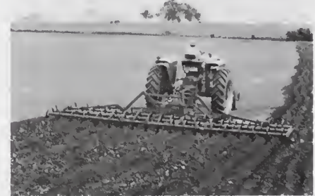
Three section tractor-mounted, spring-toothed harrow
